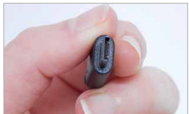
The USB Type C connector can be inserted into Vario 340 in either direction.
